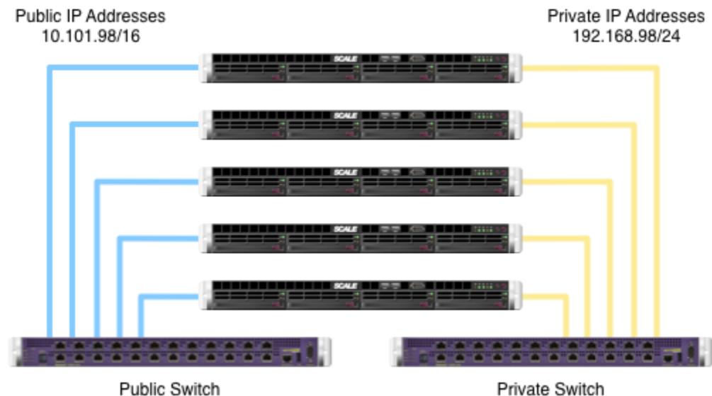
Figure 1.1. Network Cable and IP Configuration
