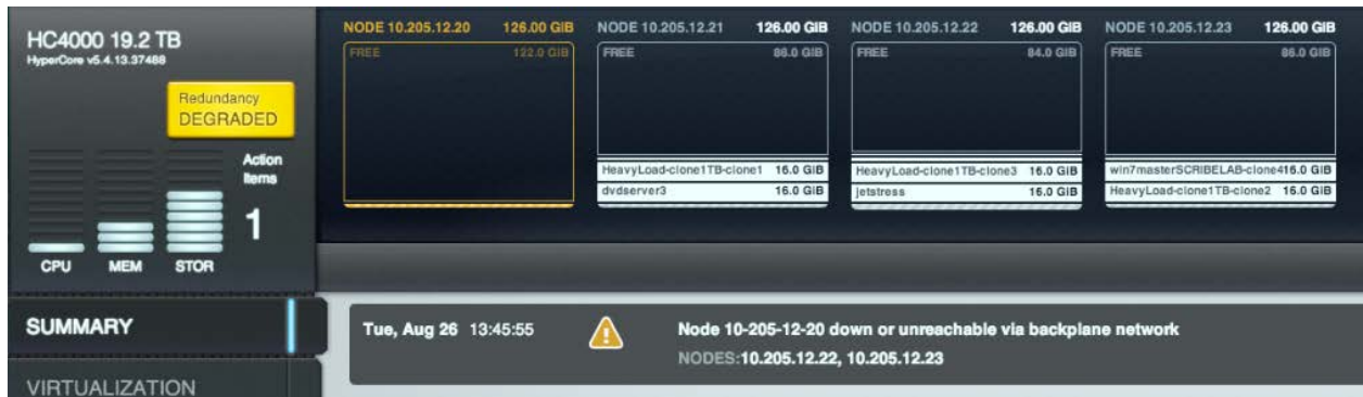
Figure 9 A four node cluster with one node down after we pulled the power cord on it.
