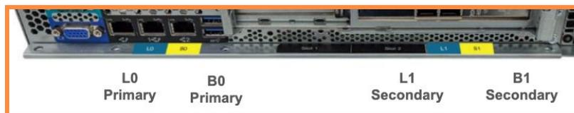
10GbE SFP+ port configuration. The 1GbE ports are permanently disabled on all 10GbE SFP+ only node series and are not functional for HC3 system use.
