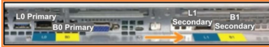
10GbE SFP+ port configuration for the HC1200 and HC1250 models. The 1GbE ports are permanently disabled on all 10GbE SFP+ only node series and are not functional for HC3 system use.
